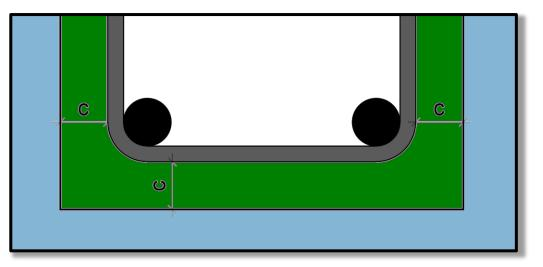
The thickness of the concrete cover *c* **must always be greater than the nominal**\* **cover layer**
