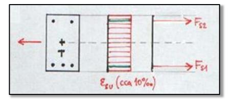
$$N_{\text{Rd},5} = F_{\text{s1}} + F_{\text{s2}} = (A_{\text{s1}} + A_{\text{s2}})f_{\text{yd}}$$
