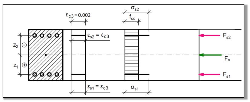
We employ the limit-force assumption which means *"assume that the*" load-bearing capacity will be equal to the acting normal force":
