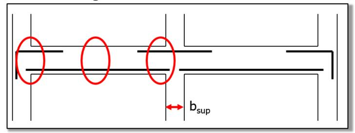
In supports, maximal values from FEM calculation should be reduced to values in the face of the column:
