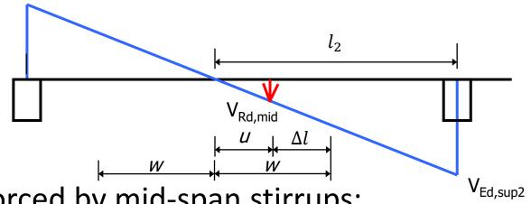
$$\frac{V_{Ed,sup2}}{l_2} = \frac{V_{Rd,min}}{u}$$
