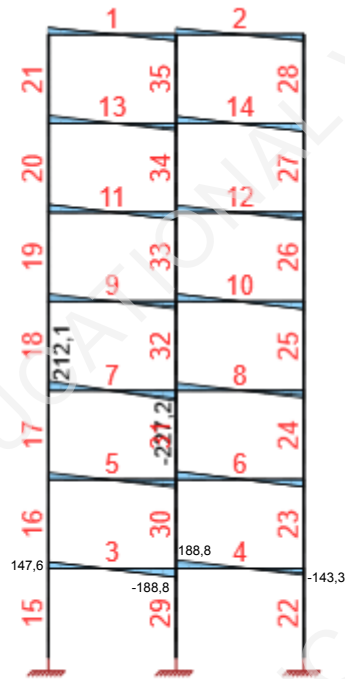
All combinations, V_z [kN], Centroidal forces
