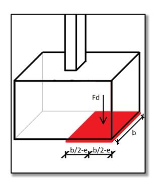
After we design the footing width, we must verify that the stress in the soil is smaller than the soil resistance:
