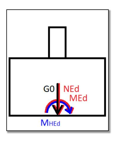
The total eccentricity of the normal force is determined by the the overall moment and overall normal force.
