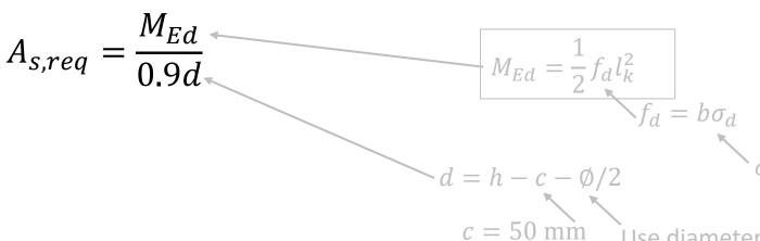
We must use the real effective loading area calculated for the RC footing! Do NOT use the value for PC footing nor the value used during the design of the footing width!
