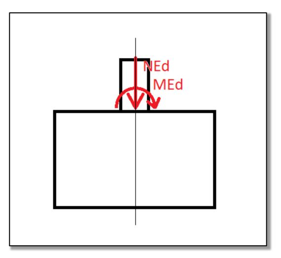
Normal force and bending moment from the upper structure acting at the base of the column.
