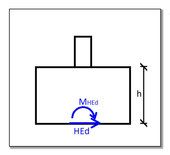
The shear force induces a bending moment at the soil level:
