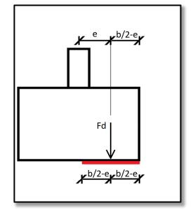
Finally, we can assess the **condition for the stress in the soil**:
