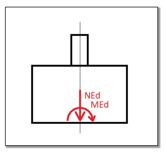
Normal force and bending moment from the upper structure acting on the soil.
