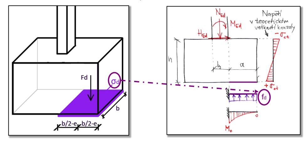
We design the height from the condition the that the most extreme tension in concrete must not exceed tensile strength of concrete
