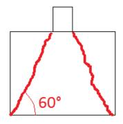
In a RC footing, the height is smaller, load-bearing angle is approximately 30° to 45°, and the **tensile stresses are big** (bigger than the tensile strength of concrete), and therefore, we must design a reinforcement to transfer the tensile stresses.
