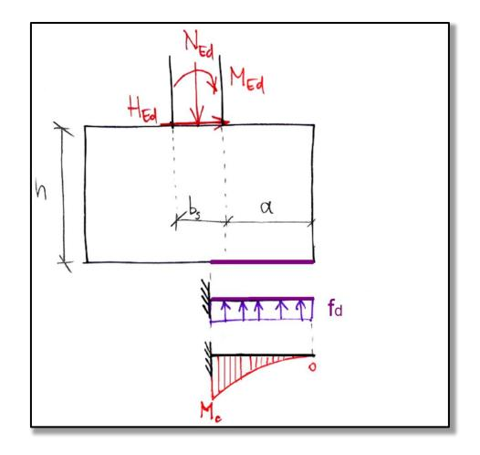
We can **choose the height** anywhere from 200 mm (puncing limit) to the height for plain concrete footing.
