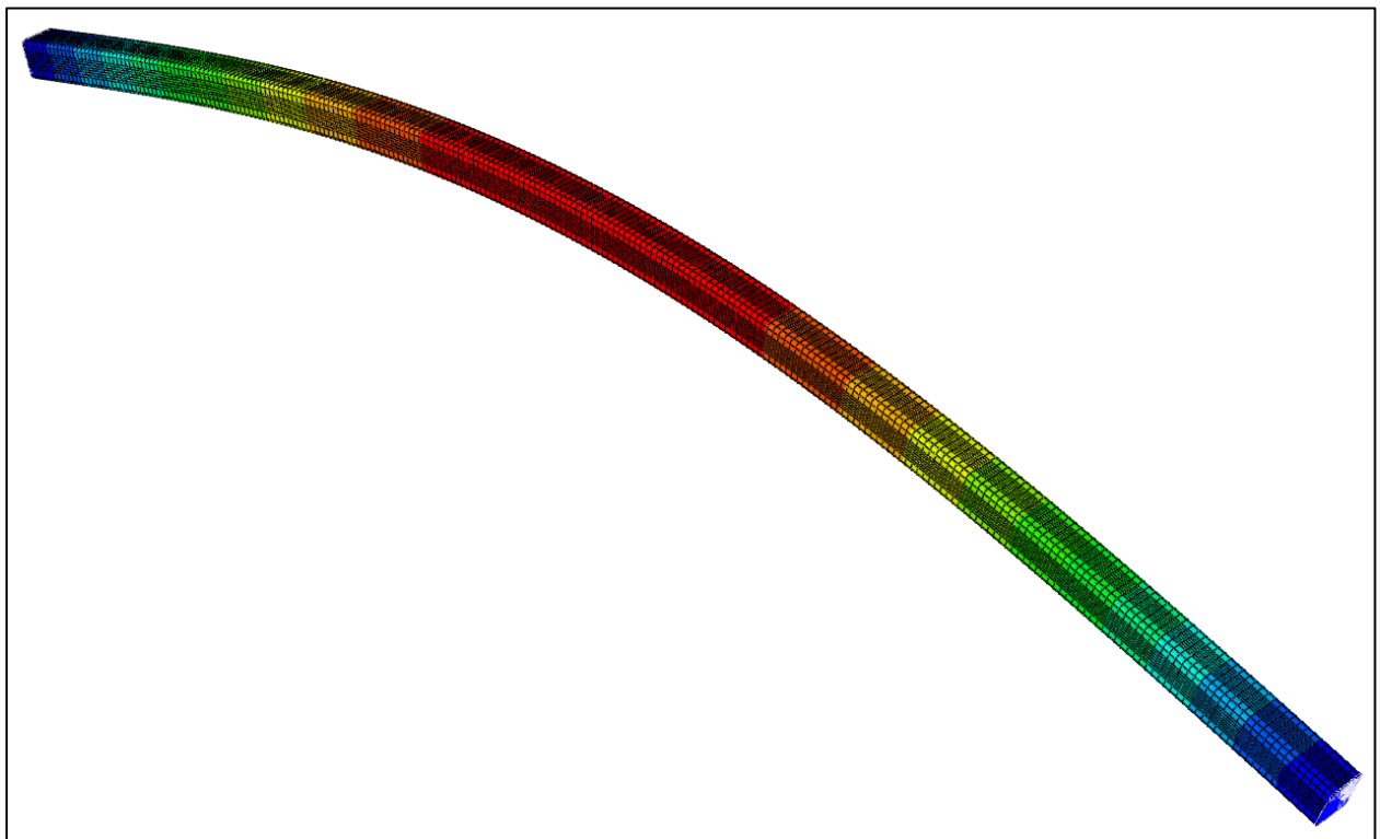
Figure 7-3 : RHS-Section global imperfection mode – Abaqus visualitation
