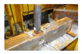
Example behaviour and curve fitting predictions of joint with RHS chord 150 x 100 x 4 mm and brace 50 x 30 x 4 mm
