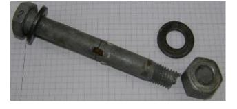
Rupture of bolt close to nut
