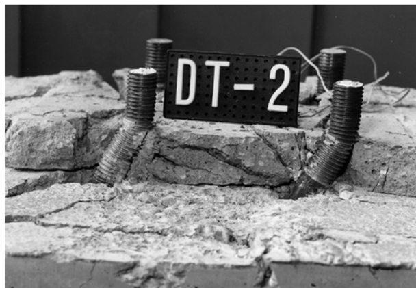
Fig. 4.20 Test specimen loaded by shear force and tensile force
