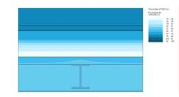
STRUCTURE OF THE ROOF THICKNESS THERMAL INSULATION 360 mm
