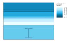
roof structure field of temperature and humidity growing steel house - family rules
