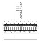
© GREENING © MATTING © ASPHALT BELTS © CATCHMENT PLATES-THERMALINSULATION THICKNESS 300 mm © VAPOR BARRIERS © CONCRETE SLABS THICKNESS 110 mm © TRAPEZOIC METAL SHEETS © STEEL BEAM-PROFILE IPE 270 © PLASTERBOARD CELLING
