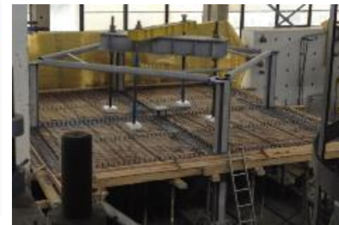
Experimental specimen before and after r.c. slab pouring
