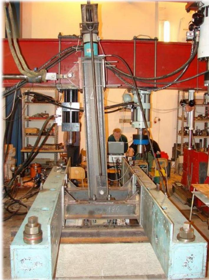
Set up in uniaxial bending
