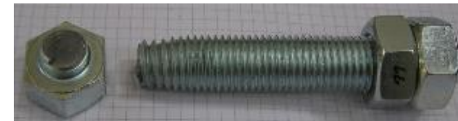
Rupture of bolt close to head
