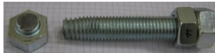
Rupture of bolt close to head
