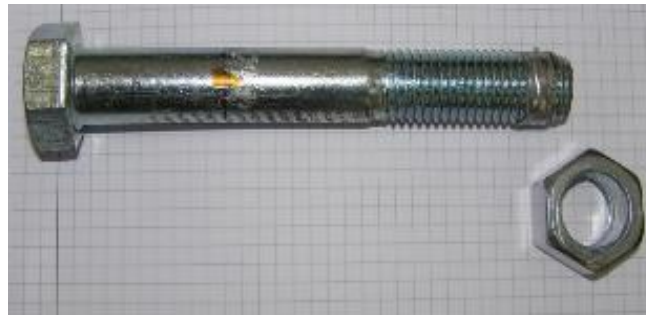
Stripping of nut threads
