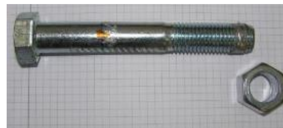
Stripping of nut threads
