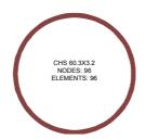
Fig. 23.13 SAFIR thermal model of space frame structural elements
