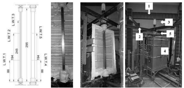
Fig. 6.2 Test set-up for CFS slender columns with restrained thermal elongation subjected to fire
