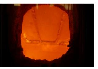
Fig. 14.6 Charring of timber at 45 mins
