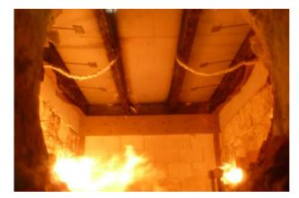
Fig. 14.5 Charring of timber at 15 mins
