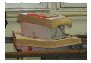
Fig. 9.6 Specimen cooled after removing from furnace chamber
