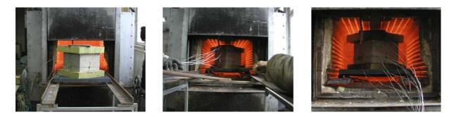
Fig. 9.3 Sample photos of a specimen 30 x 30 cm in the furnace chamber
