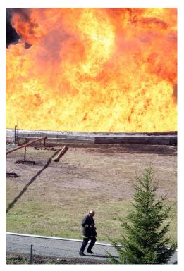
SP Fire Technology recently undertook two fire tests on 20,000 l each of denaturized ethanol and E85, respectively, in Borlänge. The tests were part of the ETANKFIRE project, the main goal of which is to provide a platform of knowledge ensuring proper investment in fire protection of ethanol storage facilities.
