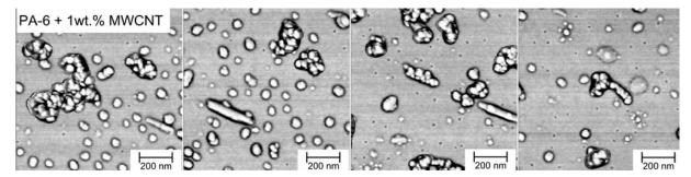
Example of aerosols emitted by Carbon-nanotube filled polyamide in cone calorimeter
