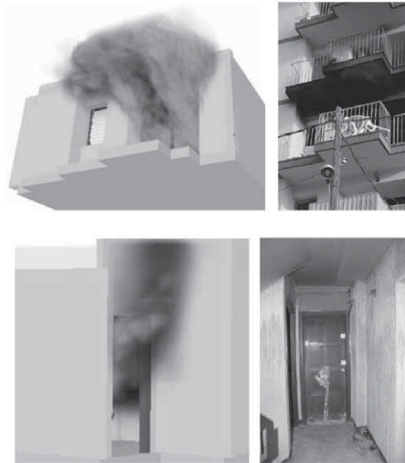
Fig. 6.3 Comparison between simulation results and real fire
