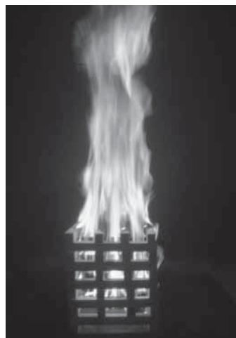
Fig. 14.7 Untreated pine crib in the test
