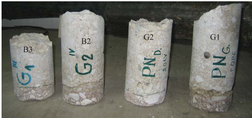
Fig. 30.3 Concrete specimens before testing
