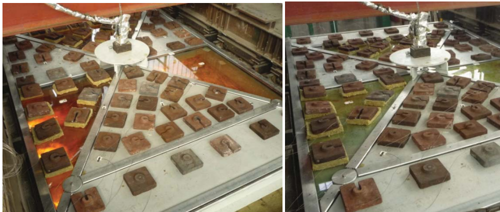
Fig. 29.19 Test model of the ceiling during the fire resistance test
