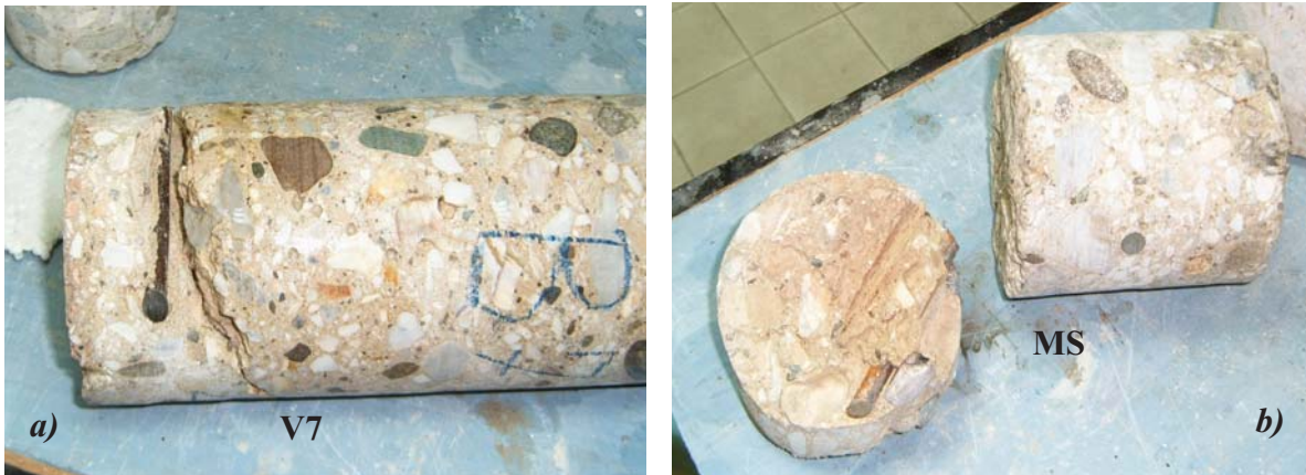
Fig. 31.3 Deterioration of surface layers of specimens
