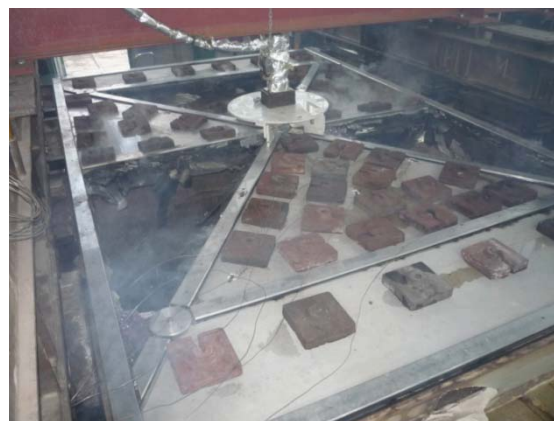
Fig. 29.20 Tested ceiling model after the fire resistance test
