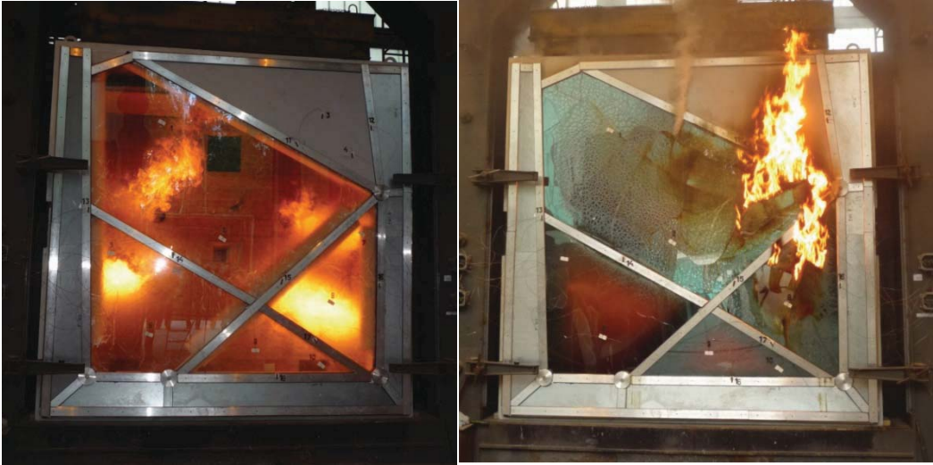
Fig. 29.16 Test model of the wall construction during the fire resistance test
