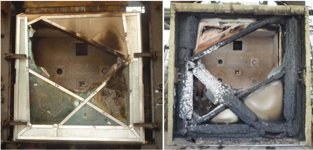
Fig. 29.17 Tested wall model after the fire resistance test (left – unexposed side, right – fire exposed side)
