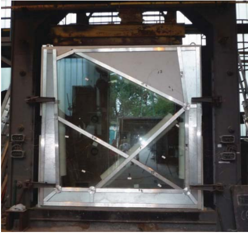
Fig. 29.15 Test model of the wall construction before the fire resistance test
