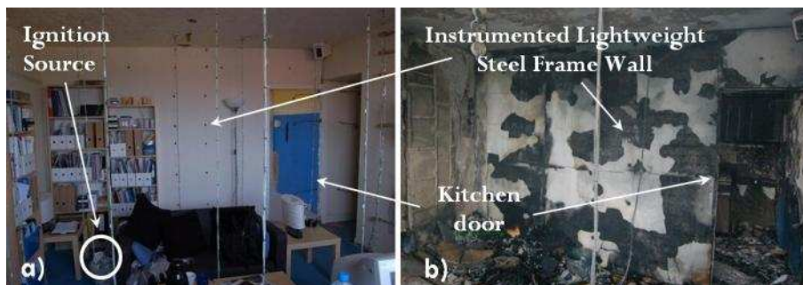
Figure 2: View of the ignition source, the sofa and nearby items in the main compartment: a) before the fire; and b) after the fire [Abecassis-Empis et al. (2008) and Rein et al. (2007)].
