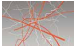
NETWORK OF FIBER CHANNELS AND CONCRETE MICROCRACKS
