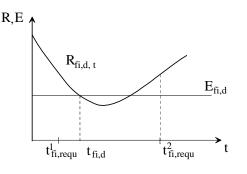
Collapse is prevented during a required period of time, t<sup>1</sup><sub>fi.reg</sub>.
