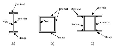
a) Rolled section; b) Hollow section; c) Welded section
