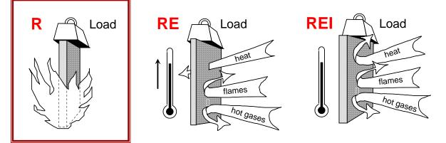
Load bearing only: mechanical resistance (criterion R)
