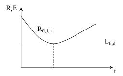
Collapse is prevented during the complete duration of the fire including the decay phase.
