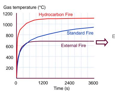
EC3 and EC9 do not use this external fire curve. A special Annex B on both Eurocodes gives a method for evaluating the heat transfer to external steelwork
