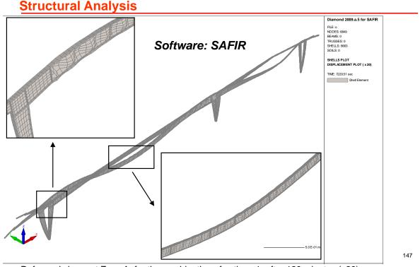
Deformed shape at Zone A, for the combination of actions 1, after 120 minutes (x20)
