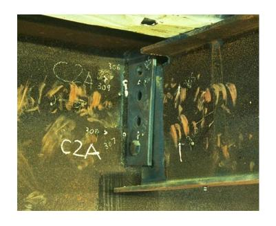
Bolt failure occurred during cooling phase
