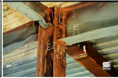
Deformed state of steel members around protected steel column
