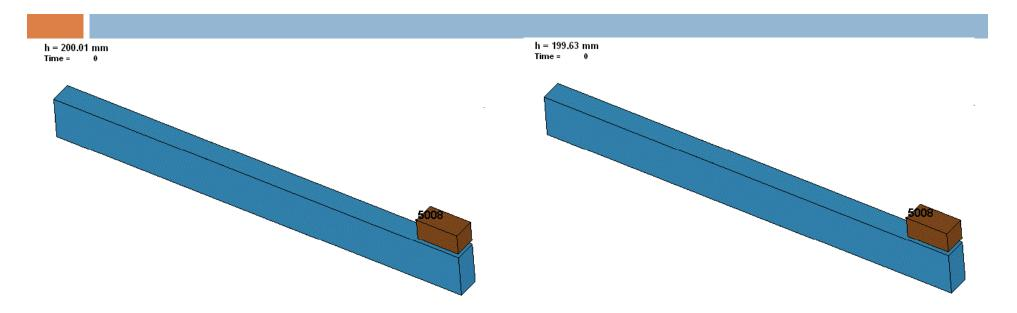
Example of on-off process –  $\Delta h = 0.38 \text{ mm} (0.19\%)$
