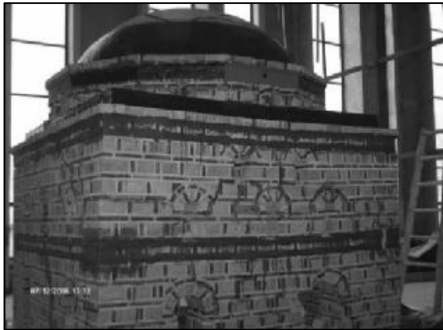
Figure 16. Damage of the model after phase 3 tests accomplishment
