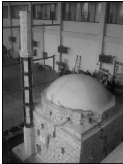
Figure 7. Repaired model and strengthened minaret after phase 1 testing
