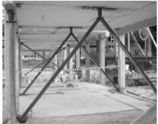
Figure 4. Experimental test on inverted Y eccentrically braced frame for rehabilitation of existing reinforced concrete frame, Mazzolani et al., 2004.
