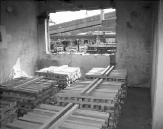
Figure 6. Fire load for the compartment fire test.
