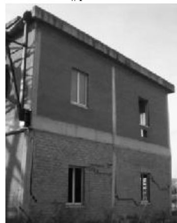
Figure 11. Damage of perimeter masonry walls at a lateral displacement of +20 cm.
