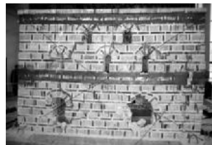
Figure 6. Mustafa Pasha Mosque model at the final damaged configuration.
