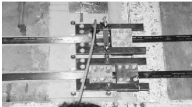
Figure 2.10. Anchoring of prestressed strips.
