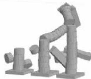
Figure 13. FEM model of an ancient Greek temple.
