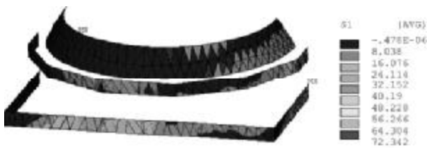
Figure 25. Tensile stress distribution on FRP sheets at the top of the dome, corresponding to the collapse load [MPa].
