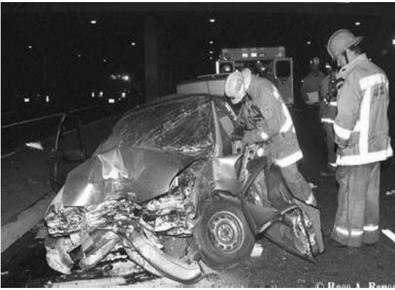
Figure 1. Energy absorbing failures of car frames achieved using the “crumple zone” design methodology
