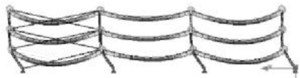
Figure 1. Car park frame with loss of a bracing
