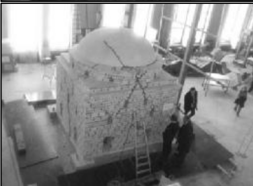
Figure 9. Damaged model after phase 2 testing
