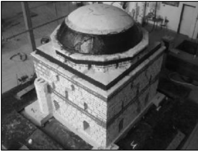
Figure 14. The strengthened model ready for testing, phase 3
