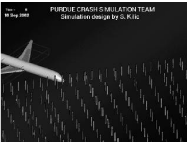
Figure 8. State of the column after impact for the initial velocity of 30.48 m/sec.
