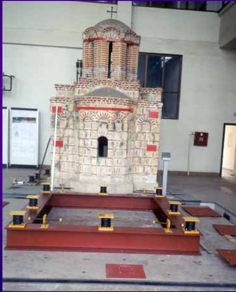
Steel structure and Isolators
