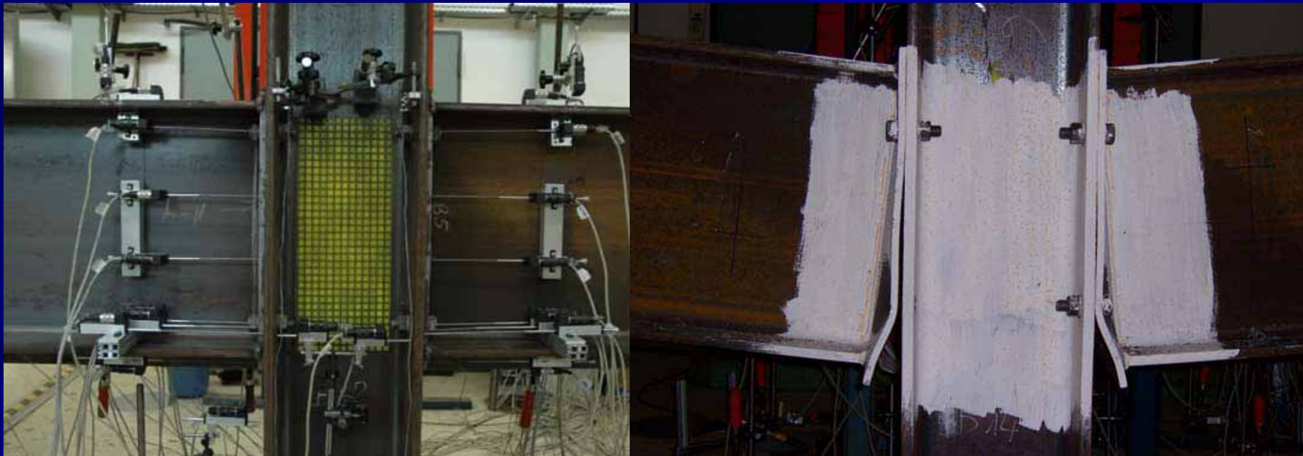
STEEL JOINTS BEFORE (left) and AFTER (right) TESTING
