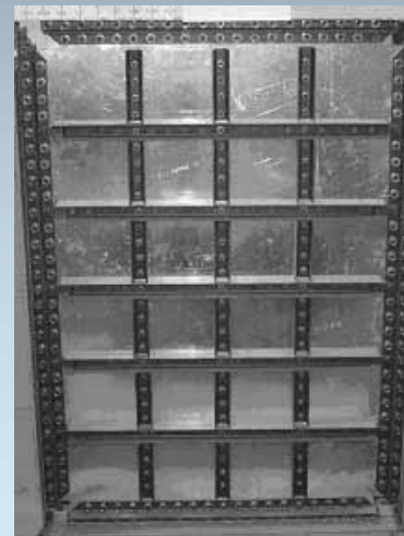
Panel type H b/t=50 (ribs: UPN50)
