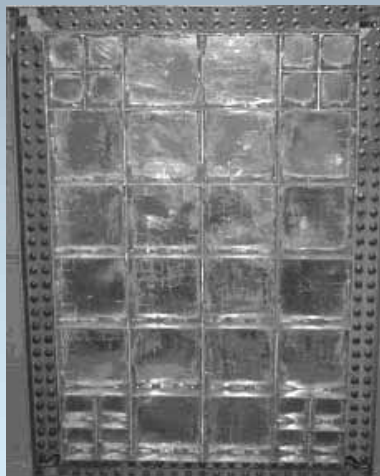
Panel type G b/t=50 (=25 in the corners)
