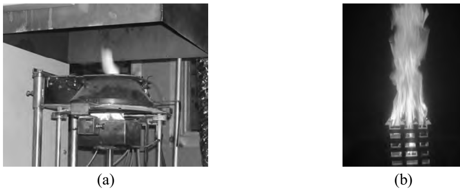
Fig. 3 (a) mdf exposed at heat flux 35 \text{ kW/m}^2 , (b) untreated mdf crib at 300 sec into the test
