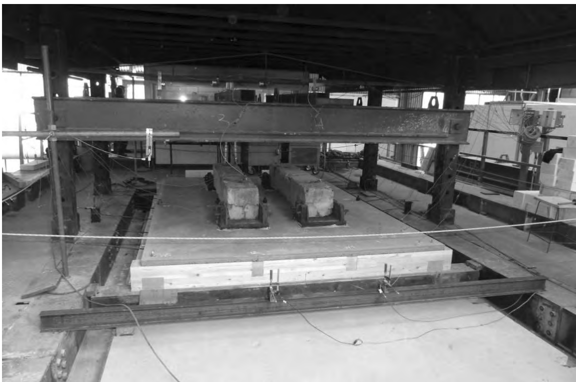
Fig. 1 Fire test set-up
