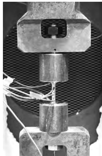
Fig. 2 Test setup for turned-down bolt specimen.
