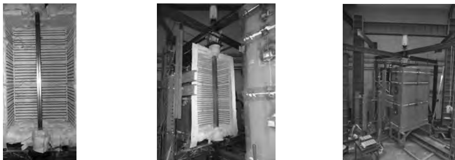
Fig. 3 Experimental set-up for CFS slender columns with thermal restrained elongation subjected to fire.
