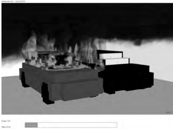
Fig. 6 Fire behaviour at the 372 nd second
