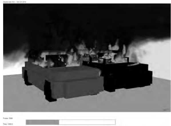
Fig. 7 Fire behaviour at the 1000 th second
