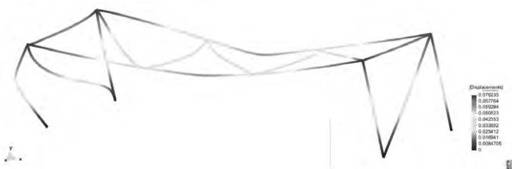
Fig. 11. Structure deformation @ 1800s, 20 mm slit for columns
