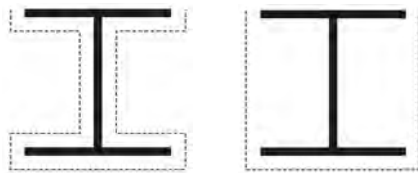
Fig. 2 The dotted line represents the heated area of the cross section. The left figure is heated with no consideration to shadow effects, whereas the right one does consider shadow effects
