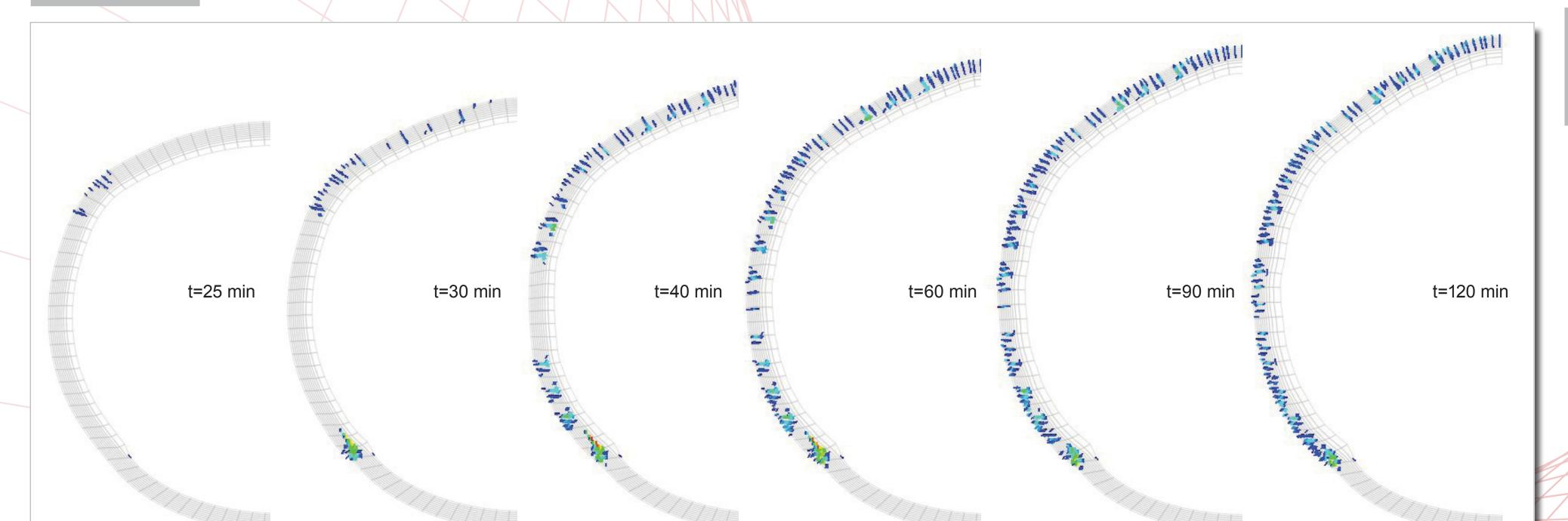
Equivalent plastic strains in concrete (left) and plastic strains in the reinforcement at the intrados (right)
