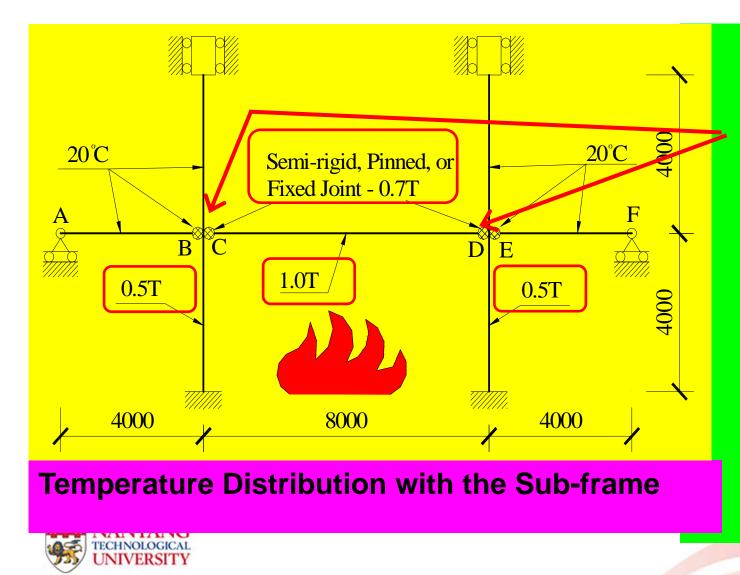
The elevated temperature profiles in the joints C & D follow the test measurements in Yuan's (2011) study
