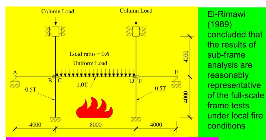
Roller supports at A & F ---> no axial restraints Fixed supports at A & F ---> with axial restraints
