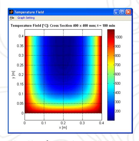
Temperature profile of a beam cross-section 400 x 400 mm<sup>2</sup> exposed to standard fire from three sides for 180 minutes
