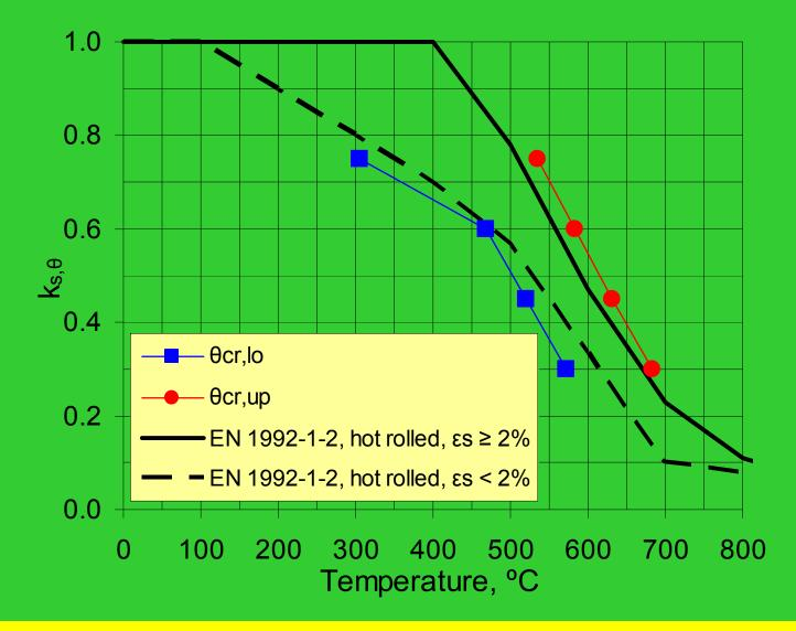
Steel strength reduction factor  $(k_{s,\theta} = f_{y,\theta}/f_{yk})$
