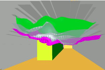
Smoke layer at the entry to the escape shaft in the 12<sup>th</sup> minute (line across the tunnel tube represents the 2.5 m height).
