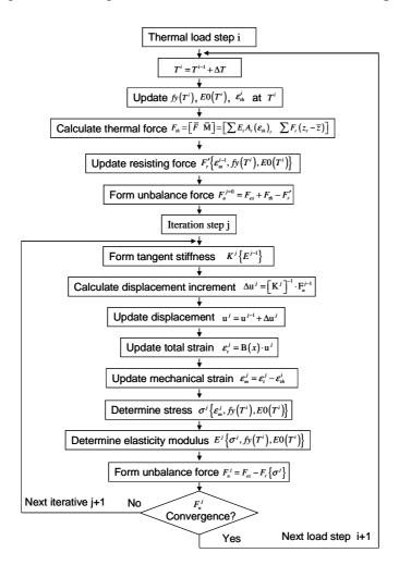
Fig. 2 Flowchart for thermo-mechanical analysis in OpenSees
