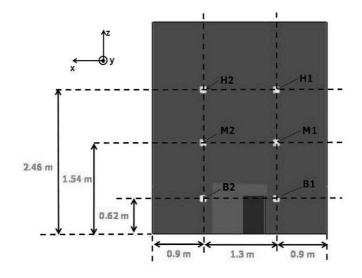
Fig. 3 Position of the plate thermometers
