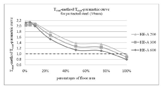
Fig. 5 Maximum steel temperature using the travelling fire method normalised by the maximum steel temperature using the parametric curve - protected steel (Jonsdottir et al. 2010).
