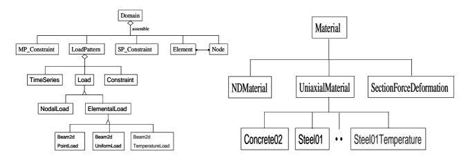
Fig. 1 Class diagram for thermal load and material in OpenSees
