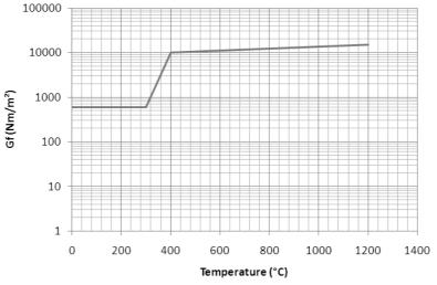
Fig. 3 Mixed fracture energy adopted in simulations
