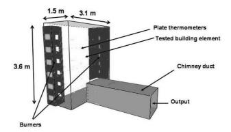
Fig. 1 Outline of the virtual furnace structure
