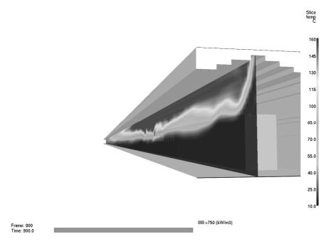
Fig. 3 Isotherm in the longitudinal cross-section of tunnel in the vicinity of fire seat in the 15<sup>th</sup> minute
