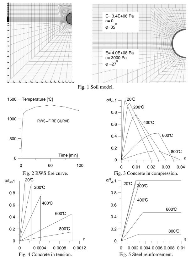
In the stress analysis, the adopted constitutive material laws are those suggested in the Eurocode 2 (EN1992-1-2). The stress-strain curve for concrete in compression is shown in Figure 3. Eurocode 2 does not give any indication for concrete in tension. In this analysis it has been chosen to use an
