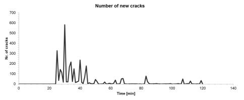
Fig 9 Crack development versus time.
