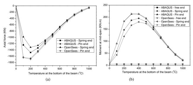
Fig. 6 Forces in the beam with different translational end restraint: (a) axial force; (b) midspan moment
