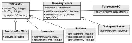
Fig. 2 Diagram representing classes for specifying boundary conditions
