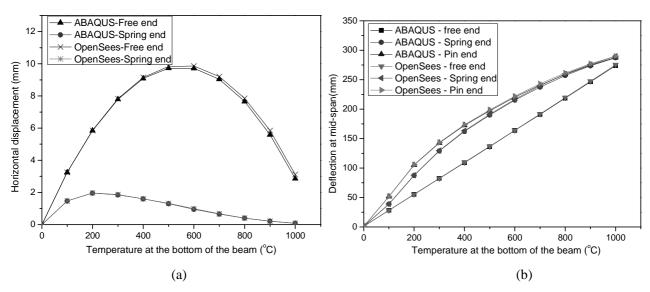
Fig. 5 Displacement of beam with different translational end restraint: (a) Horizontal displacement; (b) mid-span displacement
