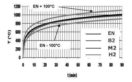
Fig. 6 Temperatures calculated by Plate Thermometers B2, M2 and H2 as function of time.
