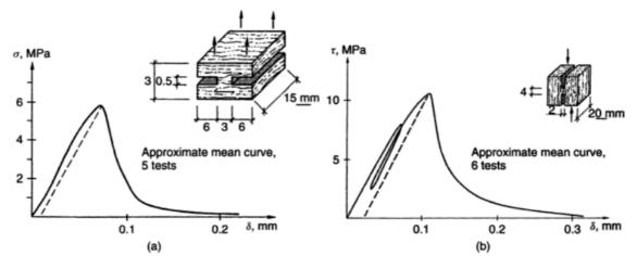
Fig. 1 Indicative fracture behaviour of timber in (a) tension and (b) shear (displacement vs. stress) after Thelanderson and Larsen (2003)
