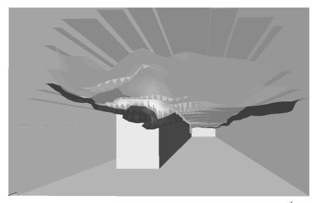
Fig. 4 Isotherms just behind the train set at 40  $^{\circ}$ C - 60  $^{\circ}$ C in the 15<sup>th</sup> minute
