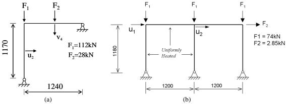
Fig. 7 Schematic of the tested steel frames (mm): (a) frame EHR3; (b) frame ZSR1
