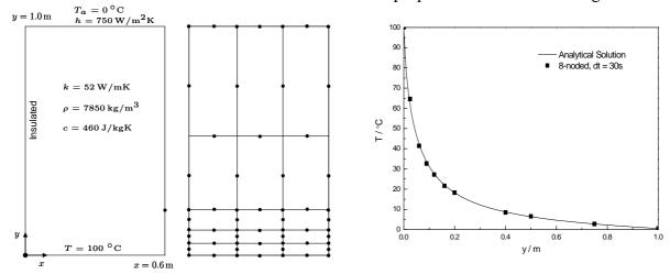
Fig. 7 Benchmark test with convection boundary condition Fig. 8 Temperature distribution along right-side boundary The steady state analytical solution suggests a strongly nonlinear temperature distribution along the right-bottom boundary. Therefore, a graded mesh shown in Fig. 7 with eight-noded elements is
