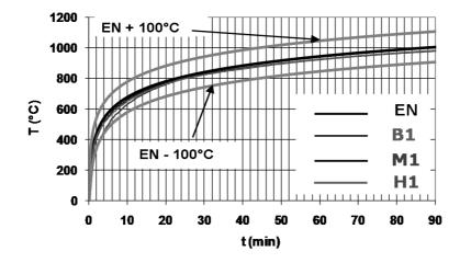
Fig. 5 Temperatures calculated by Plate Thermometers B1, M1 and H1 as function of time.
