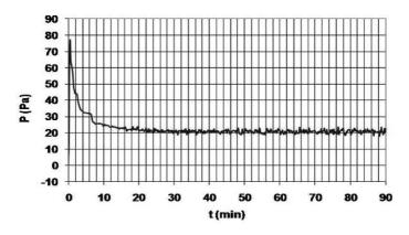
Fig. 7 Over pressure at the top of the furnace as function of time
