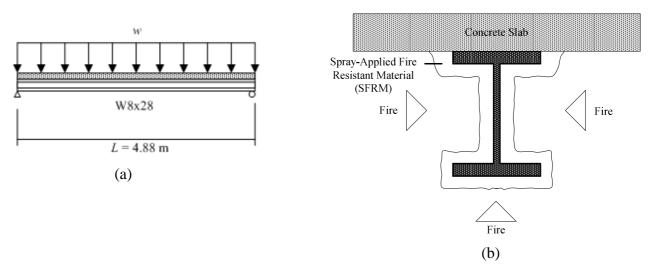
Fig. 2 Problem statement: (a) Loading and support conditions; (b) Cross-section
