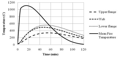
Fig. 5 Average temperatures in the steel
