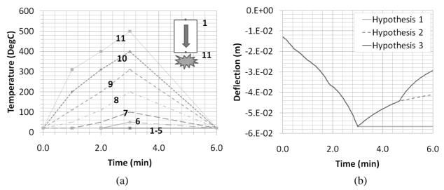
Fig. 4 Beam implementation of USRYOU and USRCST/TST subroutines: (a) Temperature profiles at integration points (b) Deflection–time plots.
