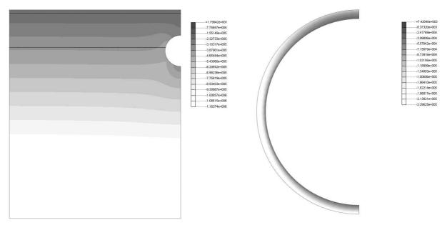
Fig. 6 Stresses in the soil and in the lining after installation of the tunnel (values in  $N/m^2$ ).
