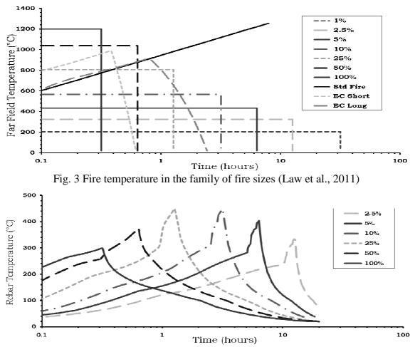
Fig. 4 Resulting temperature of the rebar in the concrete slabs for the family of fire sizes (Law et al., 2011)
