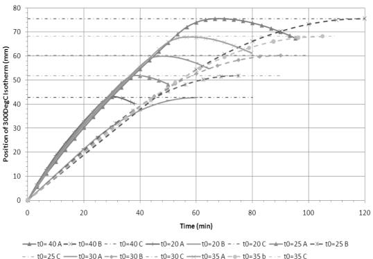
Fig. 3 Position of 300°C isotherm using modified  $k_{qtd,mod}$  (A) and EN 1995-1-2 Annex A (B). Target depth of char shown as (C).
