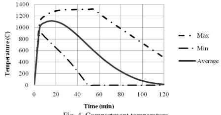
Fig. 4 Compartment temperature
