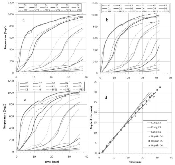
Fig. 1 (a-c) Temperature development, comparison of MCM (D), Konig (K) and EN 1995-1-2 (SFE) simulations/experiments; (d) Transient depth of char- simulation (Hopkin) versus experiment (Konig)
