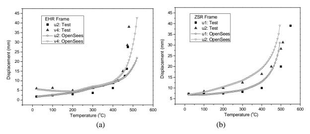
Fig. 8 Comparison between predicted and test deflection results: (a) frame EHR3; (b) frame ZSR1
