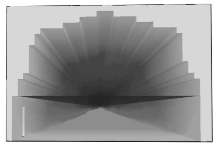
Fig. 5 Smoke layer at the entry to the escape shaft in the 12<sup>th</sup> minute (line across the tunnel tube represents the 2.5 m height)
