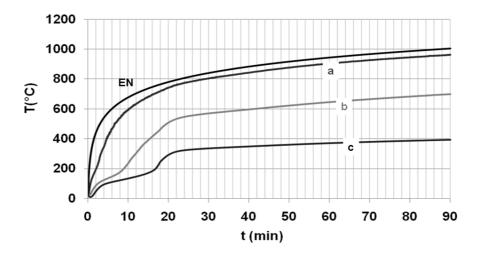
Fig. 8 Temperatures evolutions at the centre of the tested element as a function of time (EN: standard curve, a: exposed side, b: mid-thickness position, c: non-exposed side)
