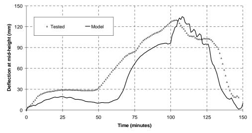
Fig. 15 Comparison of predicted deflection at mid-height of the partition with test result
