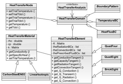
Fig. 1 Diagram for high-level classes for heat transfer module
