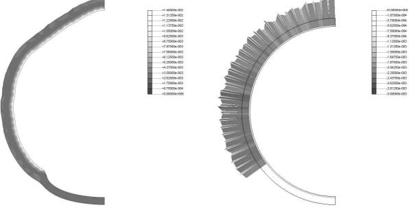
Fig. 10 Equivalent plastic strains.
