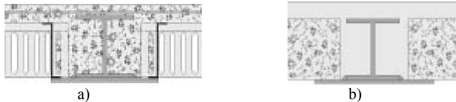
Fig. 1 Slim Floor systems a) steel beam supporting a composite floor using steel sheeting b) steel beam supporting prefabricated elements
