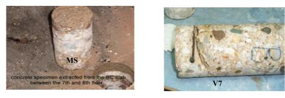
Fig. 5. Change of concrete colour and deterioration of surface layers of specimens
