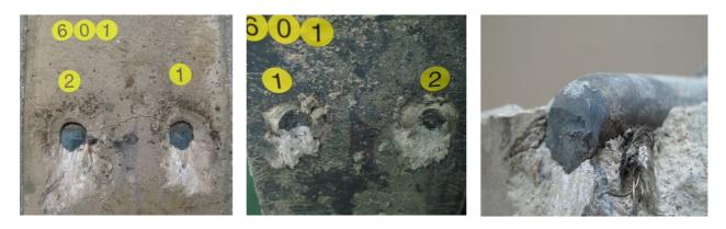
(a) Surface of concrete section (b) Surface of steel section (c) Failure of headed stud (601-2)
