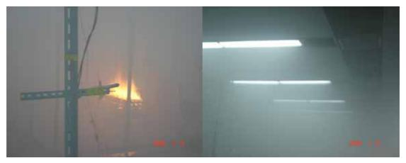
*Figure.3.* smoke movement in concourse during hot smoke test (fire source at the center of the concourse)
