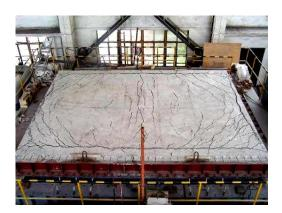
Fig.15. The cracks on the S-2 after the test
