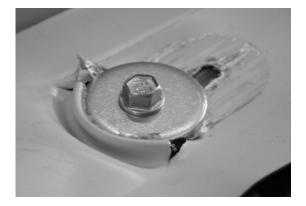
Fig. 6. The collapse mode of connection from Fig. 7. The force-displacement diagrams of the set B, temperature 200°C
