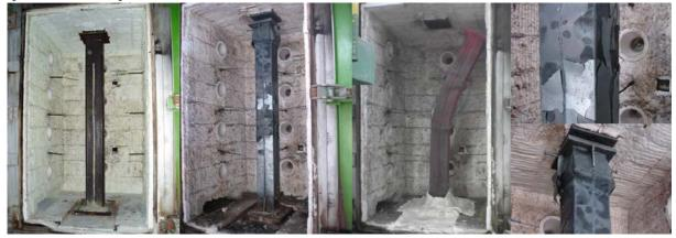
(a) A CFT column before the (b) BRH1Specimen after Experiment the Experiment (c) BRL2 Specimen after (d) Separation and column Fracture of BRH1 Specimen
