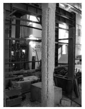
Fig. 10. Column C4 after test
