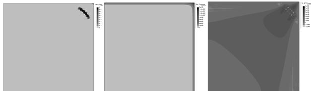
Fig. 10 Distributions of: (a) mech. dam.; (b) gas pre.; (c) stress. Perm.= $1 \times 10^{-21}$ m<sup>2</sup>; R.H.=80%; t= 200s
