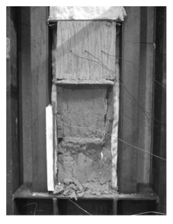
Fig .5. 1100°c unexposed face
