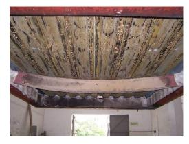
*Fig.16.* The deformation at the bottom of S-2 after the test
