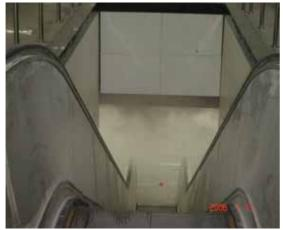
*Fig.4.* status at the mouth of the escalator under platform cold smoke test ( cold smoke source was in the center of platform )
