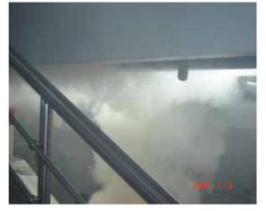
*Fig.5.* status at the mouth of the escalator under platform cold smoke test( cold smoke source was in the mouth of escalator )
