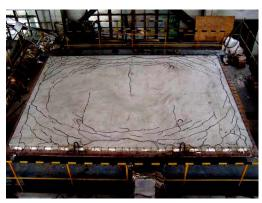
Fig.18. The cracks on S-3 after the test
