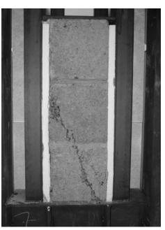
*Fig.*7. 1100°c concrete block unexposed face
