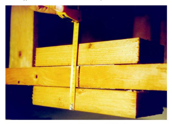
Fig.4. Detail view of overlap of a lower chord splice
