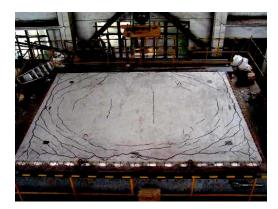
Fig.19. The cracks on S-4 after the test
