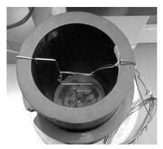
*Fig.2* Thermocouple and formwork
