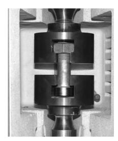
Fig. 4: Testing device bolt
