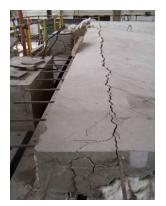
Fig.11. Cracks along the long edge
