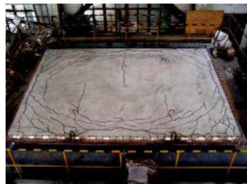
Fig.18. The cracks on S-3 after the test
