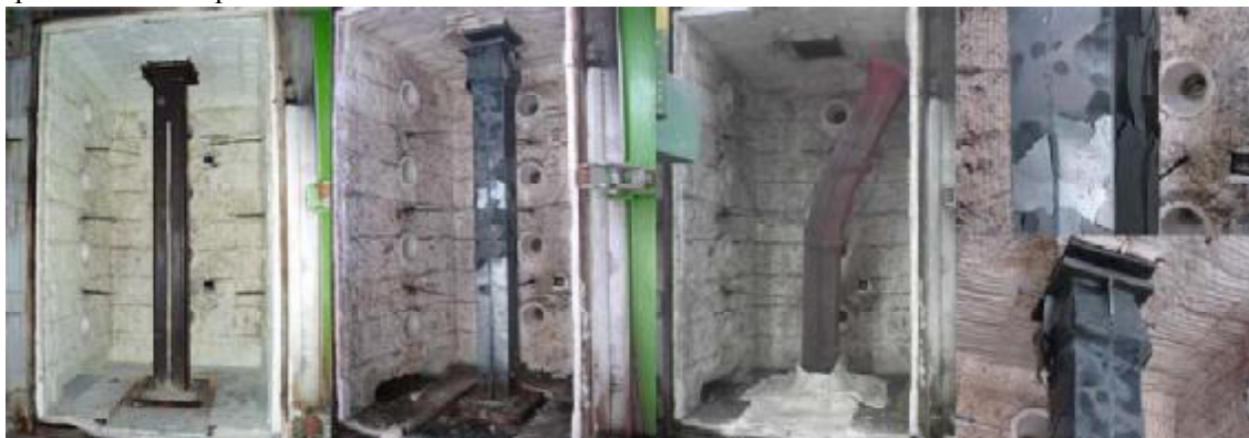
(a) A CFT column before the Experiment (b) BRH1 Specimen after the Experiment (c) BRL2 Specimen after the Experiment (d) Separation and column Fracture of BRH1 Specimen
