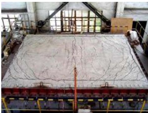
Fig.15. The cracks on the S-2 after the test
