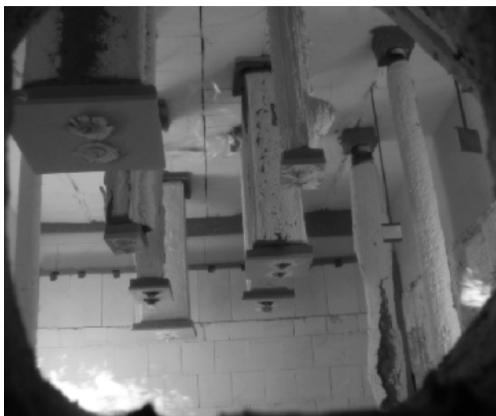
Fig. 1 The fire test of Promapaint SC, see [7]
