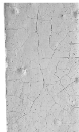
Fig. 2. Cracks on the surface of andalusite composite
