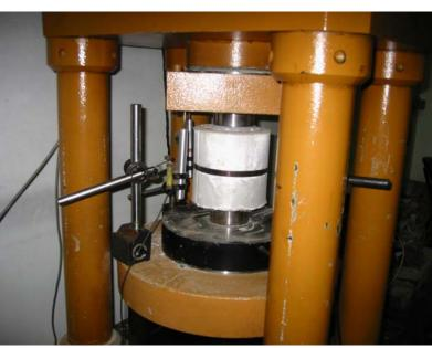
testing of pre-heated specimens
