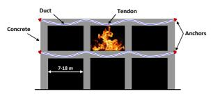
Figure 1: Single bay fire in a multi-bay structure
