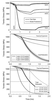
Figure 5: (a) Observed and predicted prestress relaxation for a locally-heated tendon and (b) effect of heated length ratio and (c) concrete cover at midspan on prestress relaxation during heating at 10°C/min to a predetermined temp.
