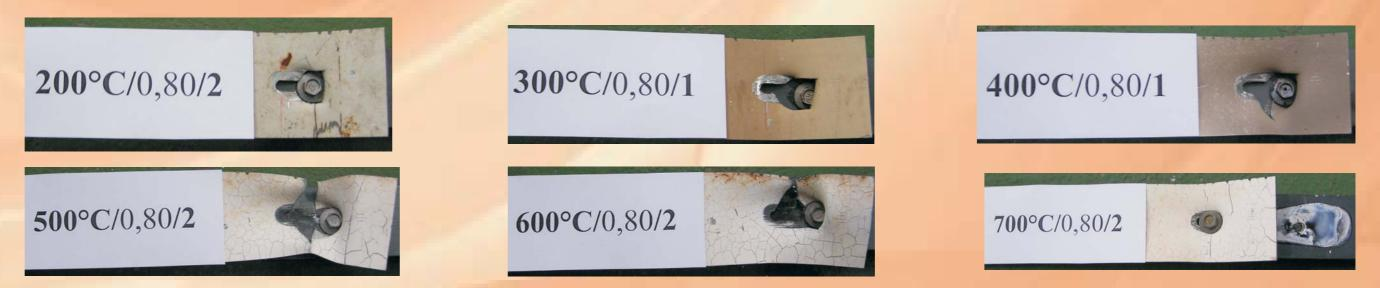
The collapse modes of the connection at specific temperatures
