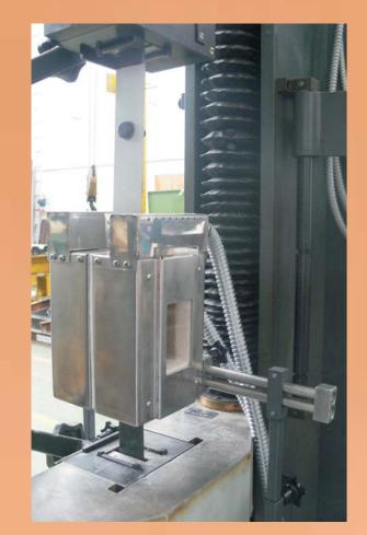
The experiments were focused on stiffness, resistance, deformation capacity and collapse mode of the connections during fire. The tested screwed connections were made by selfdrilling screws from carbon steel with marking SD8-H15-5.5x25 and trapezoidal sheets with thickness 0.75 mm and 0.80 mm. The values of material properties of used trapezoidal sheet were obtained by material experiments.
