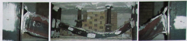
(a) Test-5, column: UC254x254x73; beam: UB178x102x19
