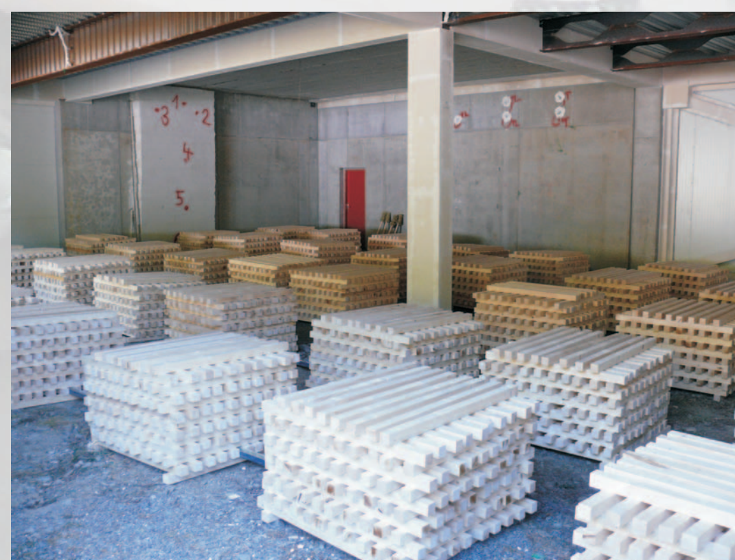
Fire load consisted of 15m 3 of wooden bars, which were evenly distributed into 50 piles
