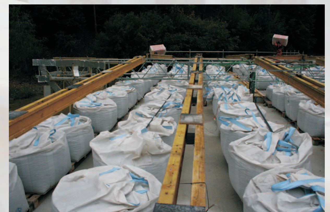
Mechanical load was represented by 78 sand bags, whose weight varied from 793 to 1087 kg
