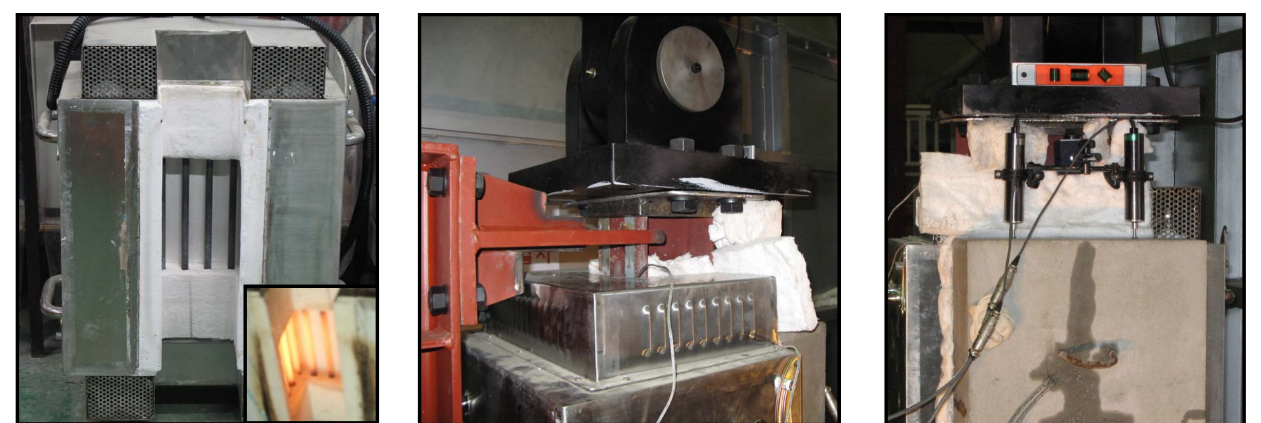
(a) Electric furnace for the test (b) Upper part of full installation (c) LVDT for slip measuring
