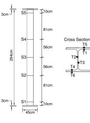
Fig. 1 - Position of the thermocouples
