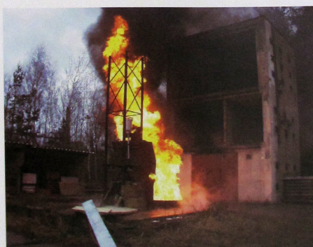
Test of components for Foam Fixed firefighting systems according to EN 13565-1
