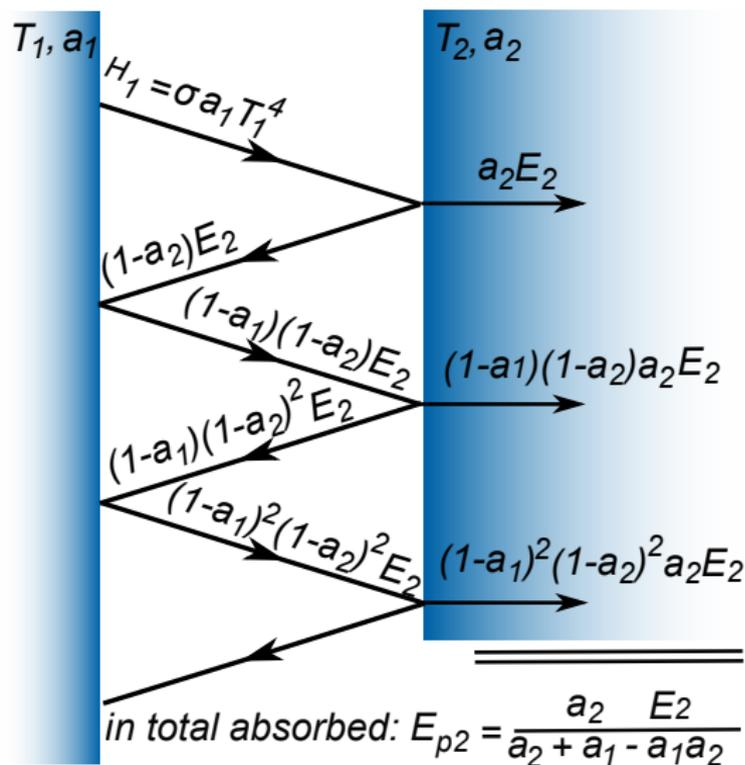
Total radiation absorbed by the right surface (sum of infinite geometric series):
