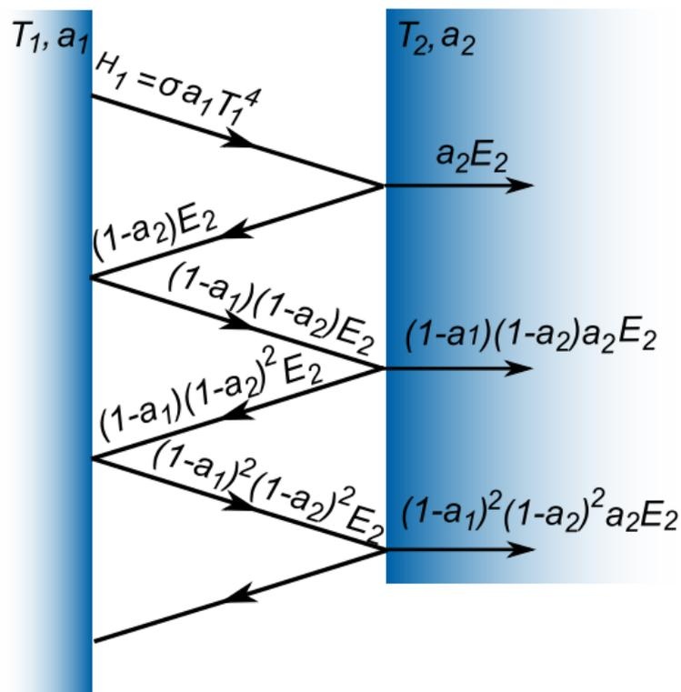
The radiation reflected from the right surface is partially reflected from the left and returned...
