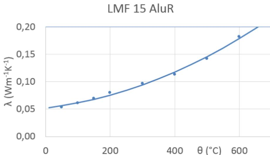
**Figure:** Heat conductivity of rock mineral wool vs. temperature
