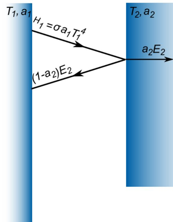
Only part of the incident radiation  $E_2$  is absorbed ( $E_{p2} = a_2 E_2$ ), the rest is reflected
