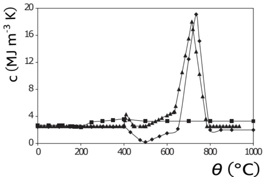
**Figure:** Concrete capacity on temperature. The capacity increase above 600  $^{\circ}\text{C}$  corresponds to the endothermic decomposition of the limestone aggregate.
