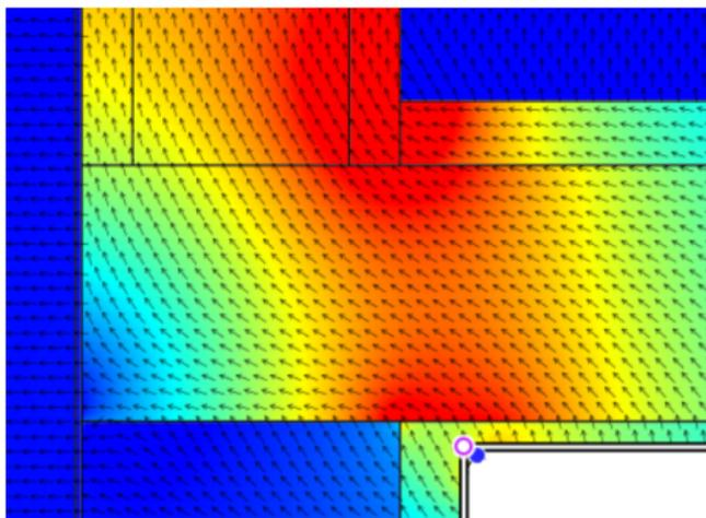
**Figure:** Heat flows in direction of temperature gradient – in corners, near thermal bridges, etc.
