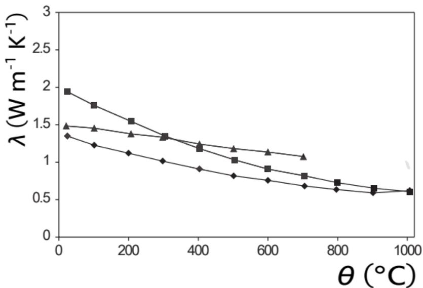
**Figure:** Heat conductivity of concrete vs. temperature
