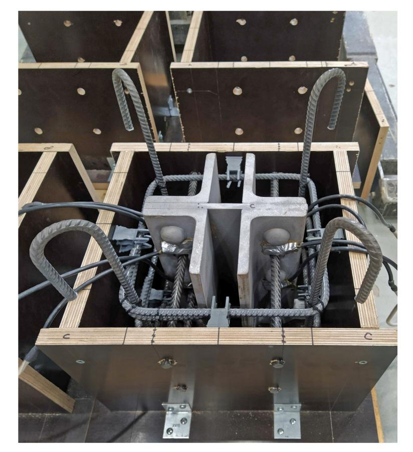
Specimen for pilot test samples before concreting
