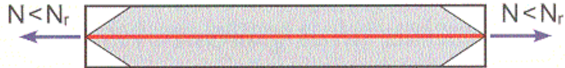
(a) Prior to formation of first crack
